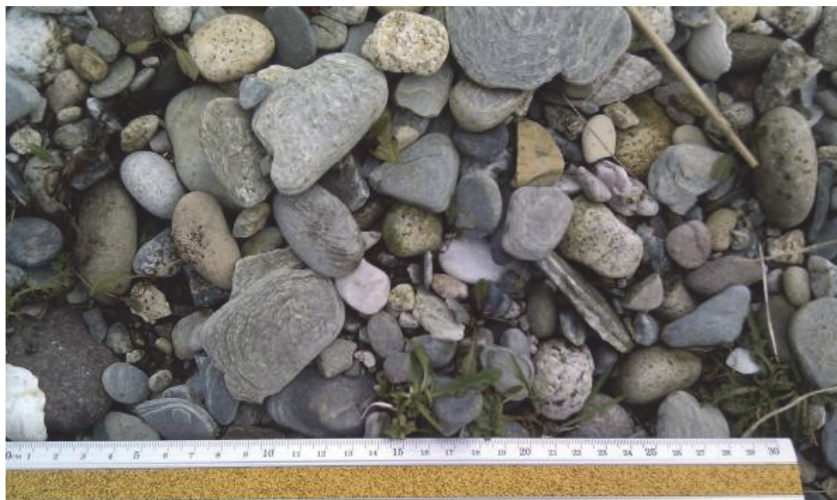
Figure 2. Recording shingle substrate size.
